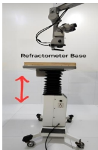
Figure 3: Repurposed ophthalmic refractometer base used as adjustable support platform.
